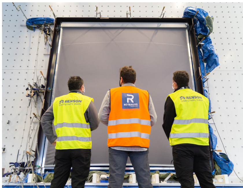
The product combination was subjected to an extensive windpressure test, performed at the test facilities of Reynaers Aluminium.
